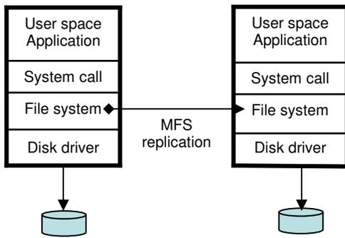
**Figure 4: Mirror File System Replication**
